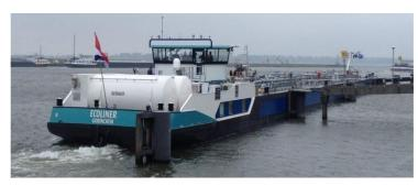
LNG-fuelled type C tanker EcoLiner developed by DAMEN within the LNG Masterplan for Rhine-Main-Danube project (2013-2015) © DAMEN
