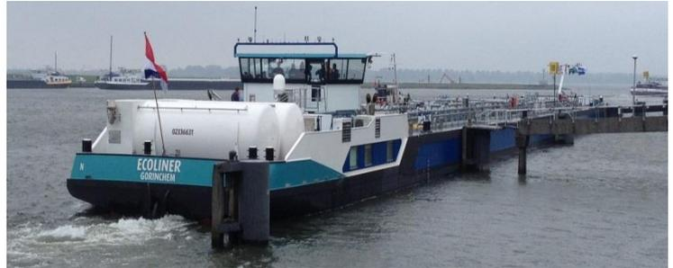
LNG-fuelled type C tanker EcoLiner developed by DAMEN within the LNG Masterplan for Rhine-Main-Danube project (2013-2015) © DAMEN
